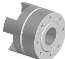
Execution with locking ring. This execution is suitable for high speed and high torque. Screws mounting from spider side. Transmissible torque depends on bore diameter.
