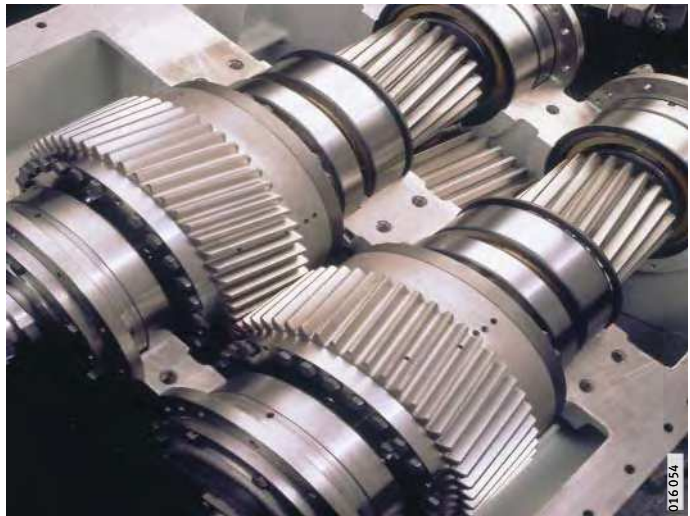
Figure 6 Rolling bearings in a cylindrical gear unit
