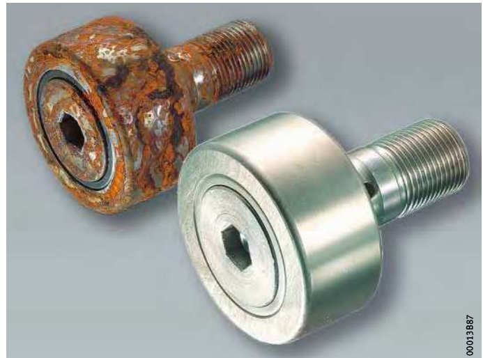
Figure 25 Uncoated and coated stud type track roller after salt spray test
