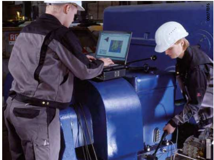
Figure 6 Vibration diagnosis as a service
