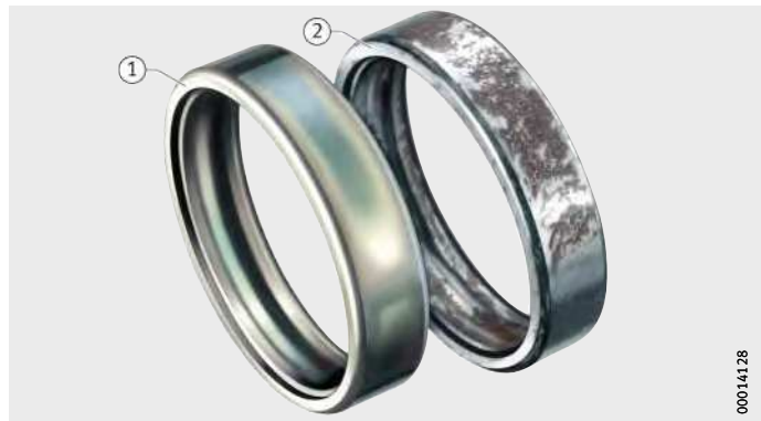
Figure 11 Bearing rings after the salt spray test
