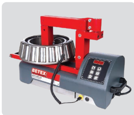
Recommended horizontal heating position
