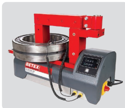
Recommended horizontal heating position
