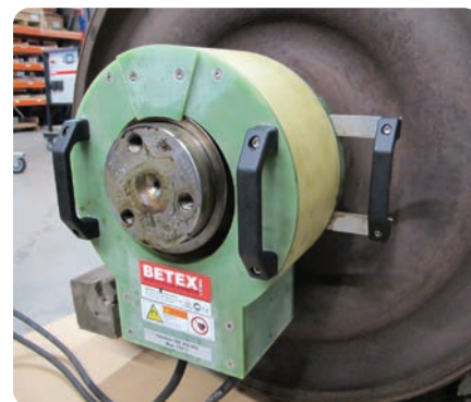
Heating bearing rings for dismantling
