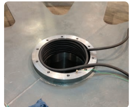
Heating a bore for bearing or shaft mounting
