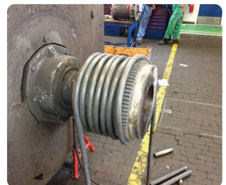
Heating a coupling for dismantling
