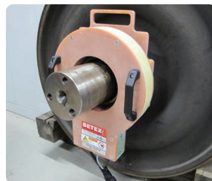
Heating labyrinth rings for dismantling
